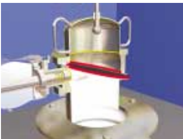
Installing wash hood on the active half and interlocking
