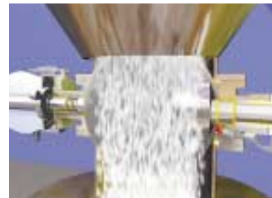
Opening of the valve and product transfer
