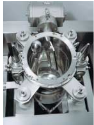
Washing station with valve opener and nozzle for cleaning of passiv valves
