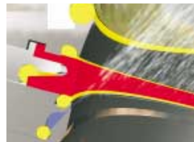
Internal air-purging of the seals
