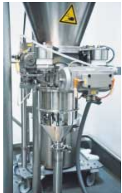
Active valve with docked drain funnel during the cleaning cycle
